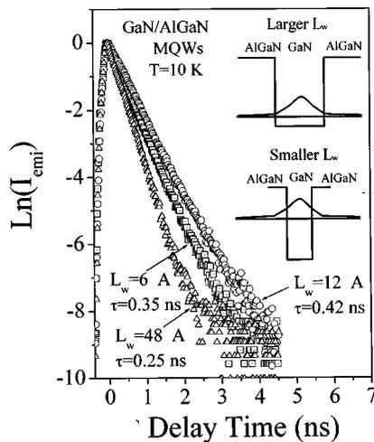
FIG. 4. PL temporal responses of the well transitions of three representative GaN/Al<sub>x</sub>Ga<sub>1-x</sub>N MQWs with  $L_w = 6, 12,$  and  $48 \text{ \AA}$  measured at 10 K. The inset shows the electron wave function distribution in GaN/Al<sub>x</sub>Ga<sub>1-x</sub>N MQWs with large and small well widths.
