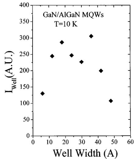
FIG. 2. The integrated well emission intensity vs well width for the GaN/Al<sub>x</sub>Ga<sub>1-x</sub>N MQWs measured at 10 K.
