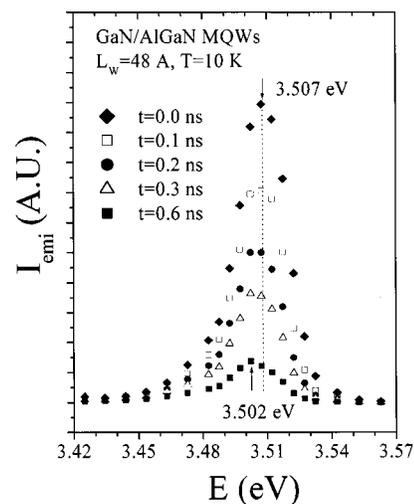
FIG. 3. Time-resolved PL spectra of the 48 Å well GaN/Al<sub>x</sub>Ga<sub>1-x</sub>N MQW sample, showing a total redshift with delay time of about 5 meV.
