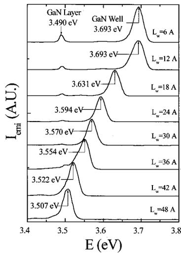
FIG. 1. PL spectra of GaN/Al<sub>x</sub>Ga<sub>1-x</sub>N MQW samples with well width varying from 6 to 48 Å and a fixed barrier width of 50 Å measured at 10 K.
